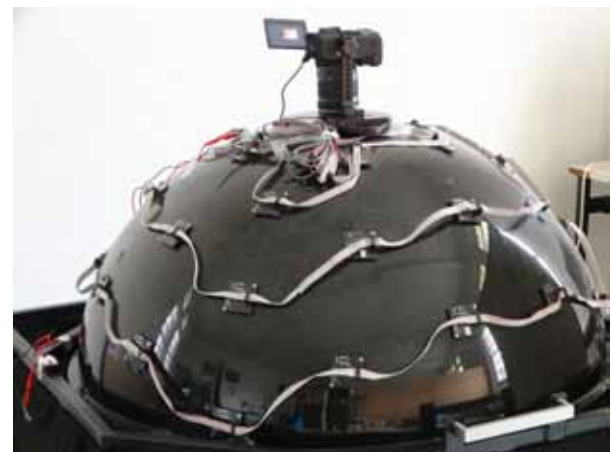
Figure 1: The multi-light illuminations dome for capturing RTI images at the AIA.
