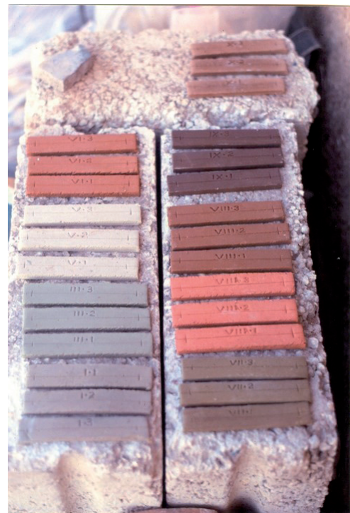
Figure 7: Test bars of the different clay samples.
