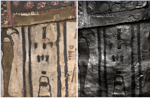
Figure 7: Detail of the surface of the chest cartonnage. Left, a visible light photograph, and Right, a specular enhanced image captured using Reflectance Transformation Imaging showing surface undulations. Image: Grimwade Conservation Services, 2017.
