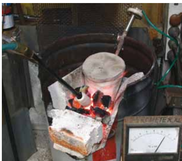
Figure 21: The experimental set-up showing the blowpipe nozzle directed into the crucible over the barrier with the thermocouple displaying a temperature of 1140°C. From Davey and Edwards (2007).
