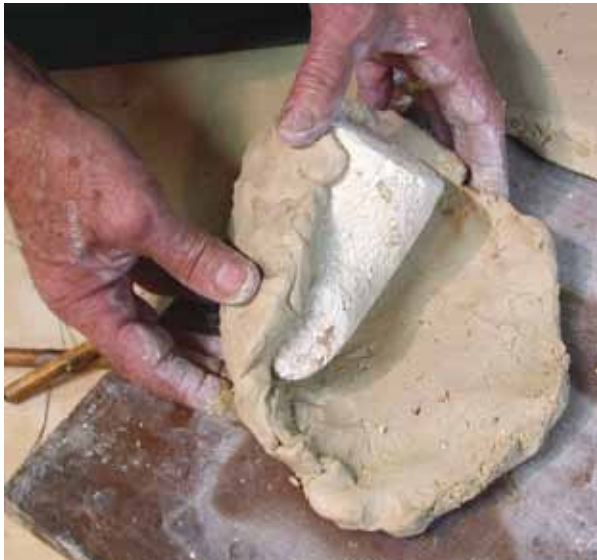
Figure 20: The forming of the crucible using a horn-shaped pattern. From Davey and Edwards (2007).
