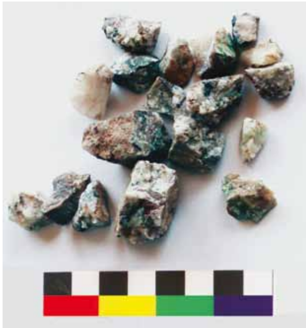
Figure 16: Smelter feed from Elkab. The sample consists of green malachite in a quartz host rock with a brown mineral formed from decomposed pyrite-arsenopyrite. Courtesy of the Belgian Archaeological Mission to Elkab, used with permission.
