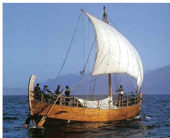
Figure 1: Kyrenia II , a replica of a fourth-century BC merchant ship found near Kyrenia , Cyprus, seen here sailing to windward in light air. The wind is coming directly toward the camera. Image: courtesy Kyrenia Shipwreck Collection Restoration Program .
